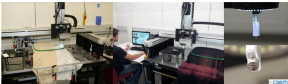
Figure 15: Assembly machine for automatic placement of dies and stretchable interposers. Source: http://www.pasta-project.eu/
